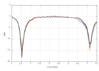
• Coupling between two adjacent elements in E-plane.
