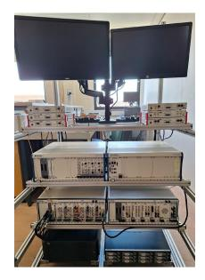
National Instruments (NI) Software Defined Radios (SDRs) are used for digital baseband generation, RF up/down-conversion, IF sampling, etc. Tx and Rx SDR modules include
