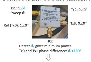
Similar method to find  $\vartheta_2$  for Tx2 and  $\vartheta_3$  for Tx3
